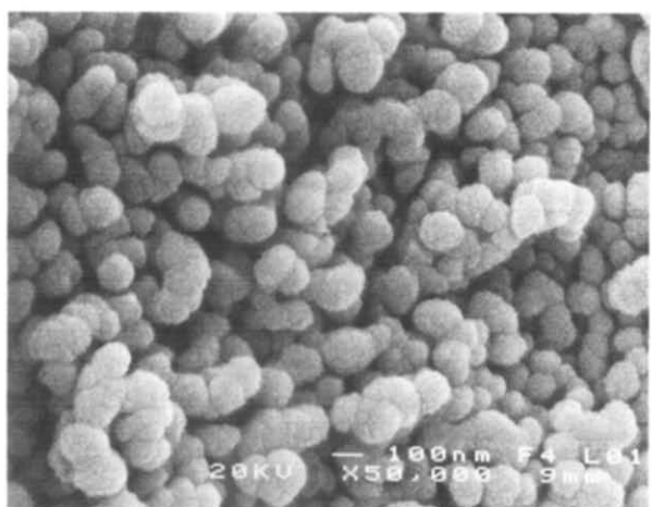
Fig. 5. SEM micrographs of (a) BaSnO_2(O_2) \cdot 3H_2O , (b) powder obtained after calcination of BaSnO_2(O_2) \cdot 3H_2O at 550^\circ C for 1 h and (c) BaSnO_3 obtained after calcination of BaSnO_2(O_2) \cdot 3H_2O at 900^\circ C for 1 h.
